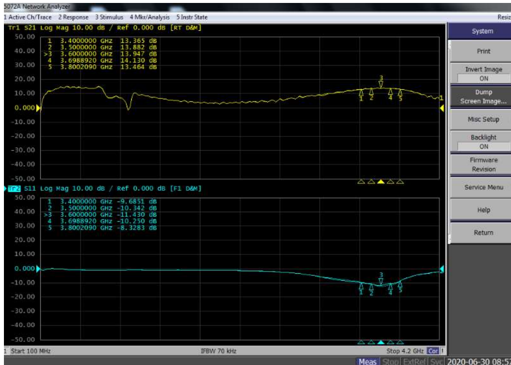
Figure 4: S11 / S21 output from network analyzer
