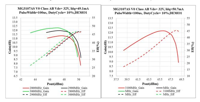
Figure 1. Power Gain and Drain Efficiency as Function of Pulse Output Power
