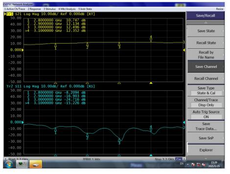
Figure 2. Network analyzer output S11/S21 (VDS=32V IDQ=380mA VGS=3.1V)
