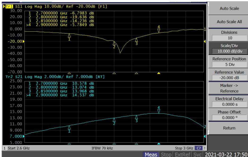
Figure 1. Network analyzer output S11/S21 ( V_{DS}=28V, I_{DQ}=250mA, V_{GS}=3.75V )
