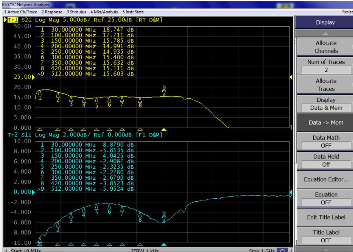
Figure 1: Network analyzer output S11/S21 at 28V Idq=500mA
