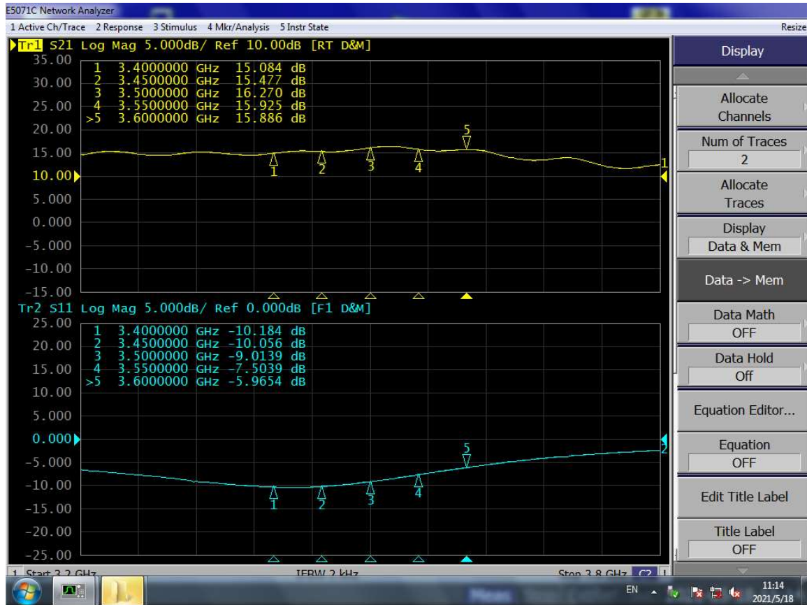
Figure 3. Network Analyzer result S11 and S21 (3400MHz~3600MHz)
