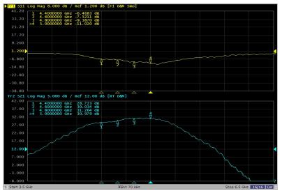
Figure 4. Network analyzer output, S11/S21
