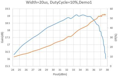
\_\_\_\_\_2000MHz\_Gain (dB) \_\_\_\_\_\_2000MHz\_Eff (%)
