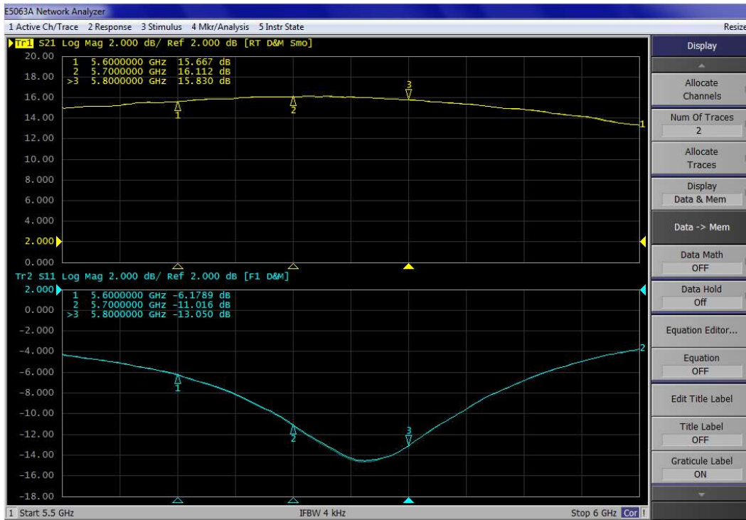
Figure 4: S11/S21 output from Network analyser (VDS= 50V, IDQ=100 mA Vgs =-3.08V)
