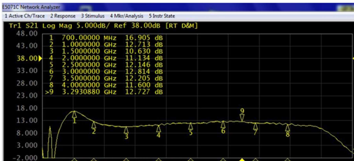
Figure 3: Network analyzer output, S21 (VDS=50V VGS=-3.31V IDQ=55mA)
