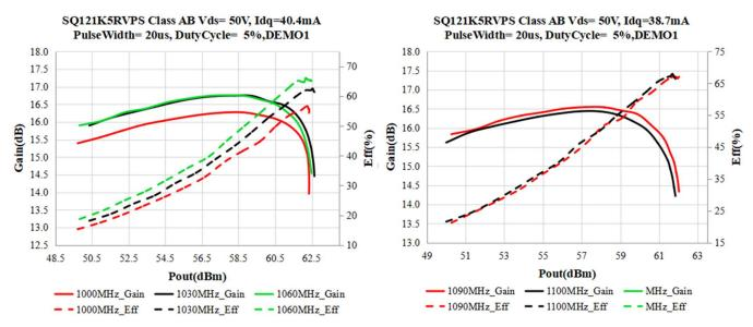
Figure 2. Power Gain and Drain Efficiency as Function of Pulse Output Power (1030-1090MHz)
