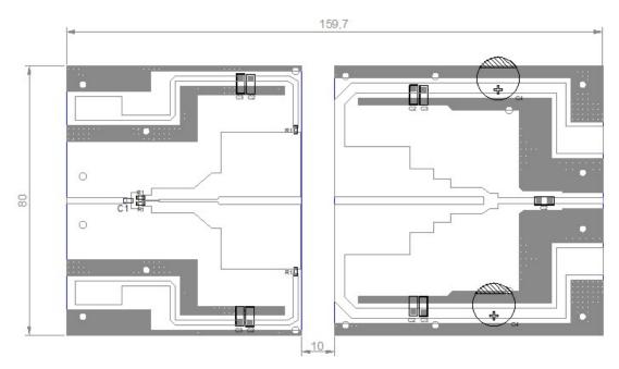
Figure 1. Test Circuit Component Layout
