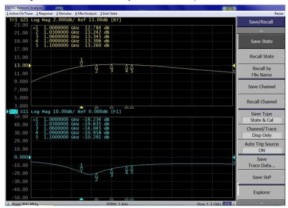
Figure 3. Network analyzer output S11/S21
