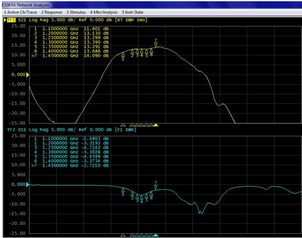
Figure 1. Network analyzer output S11/S21 ( V_{ds}=32V I_{dq}=1A V_{gs}=2.8V )
