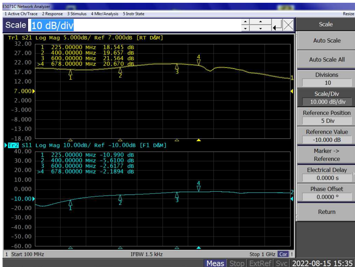
Figure 4. Network analyzer output S11/S21
