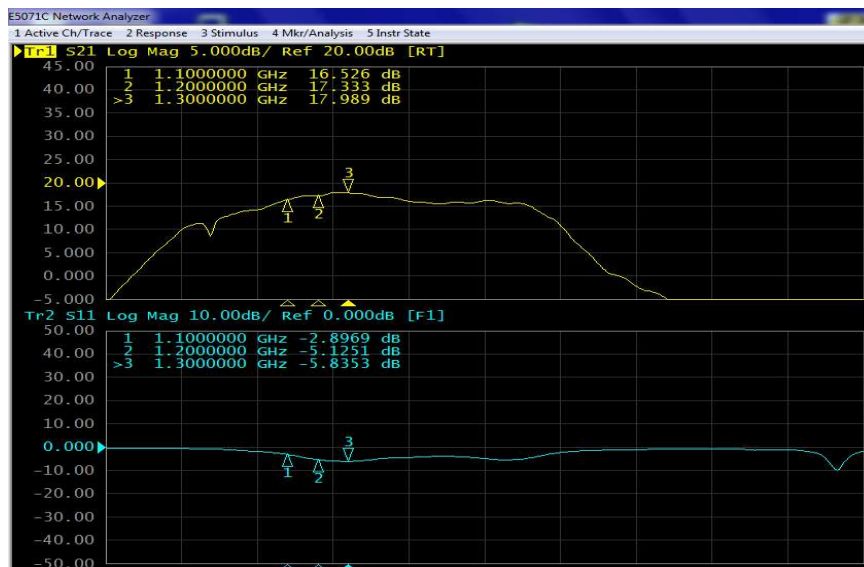
Figure 3: Network analyzer output, S11 and S21 ( VDS=28V VGS=-2.61V IDQ=500mA)
