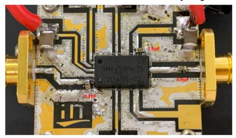
Figure 1. Test Circuit Component Layout
