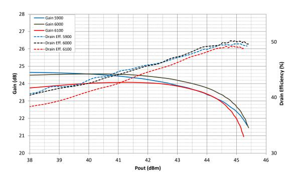
Figure 2. Power Gain and Drain Efficiency as Function of Pulsed CW Output Power
