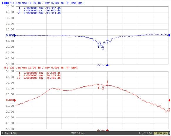
Figure 3. Network analyzer output, S11/S21
