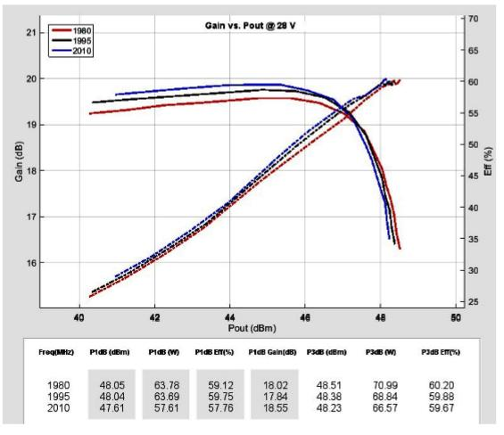
Figure 2. Power Gain and Drain Efficiency as function of Power Out
