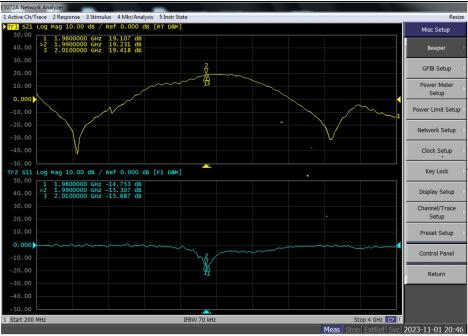
Figure 3. S11 and S21 of Network analyzer output
