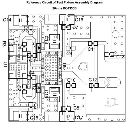
Figure 2. Test Circuit Component Layout
