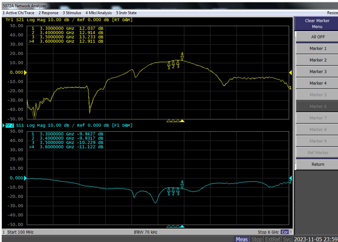
Figure 4: Network analyzer output, S11 and S21
