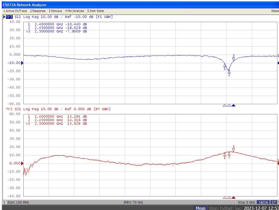
Figure 5: Network analyzer output S11/S21
