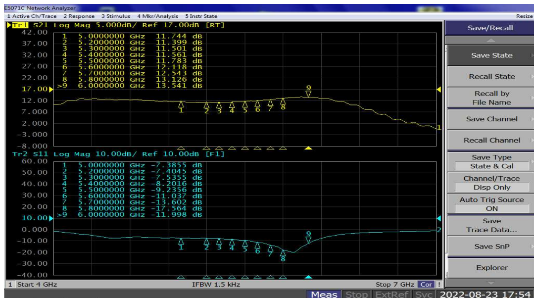
Figure 4: Small signal gain and return loss Vs Frequency V_{gs} = -2.59V , V_{ds} = 28V , I_{dq} = 500mA , input power = 0dBm
