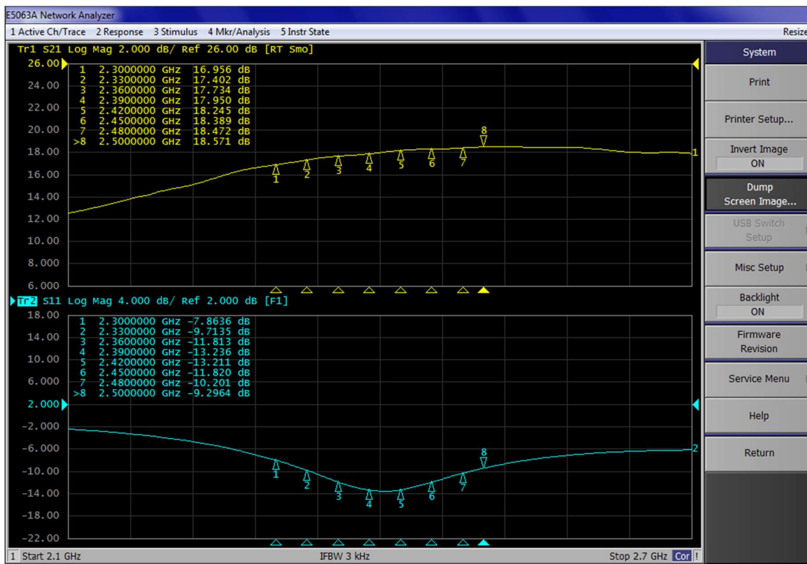
Figure 2: S11/S21 output from Network analyser ( V_{DS}=50\text{V} , I_{DQ}=500\text{mA} V_{gs}=-3.26\text{V} )
