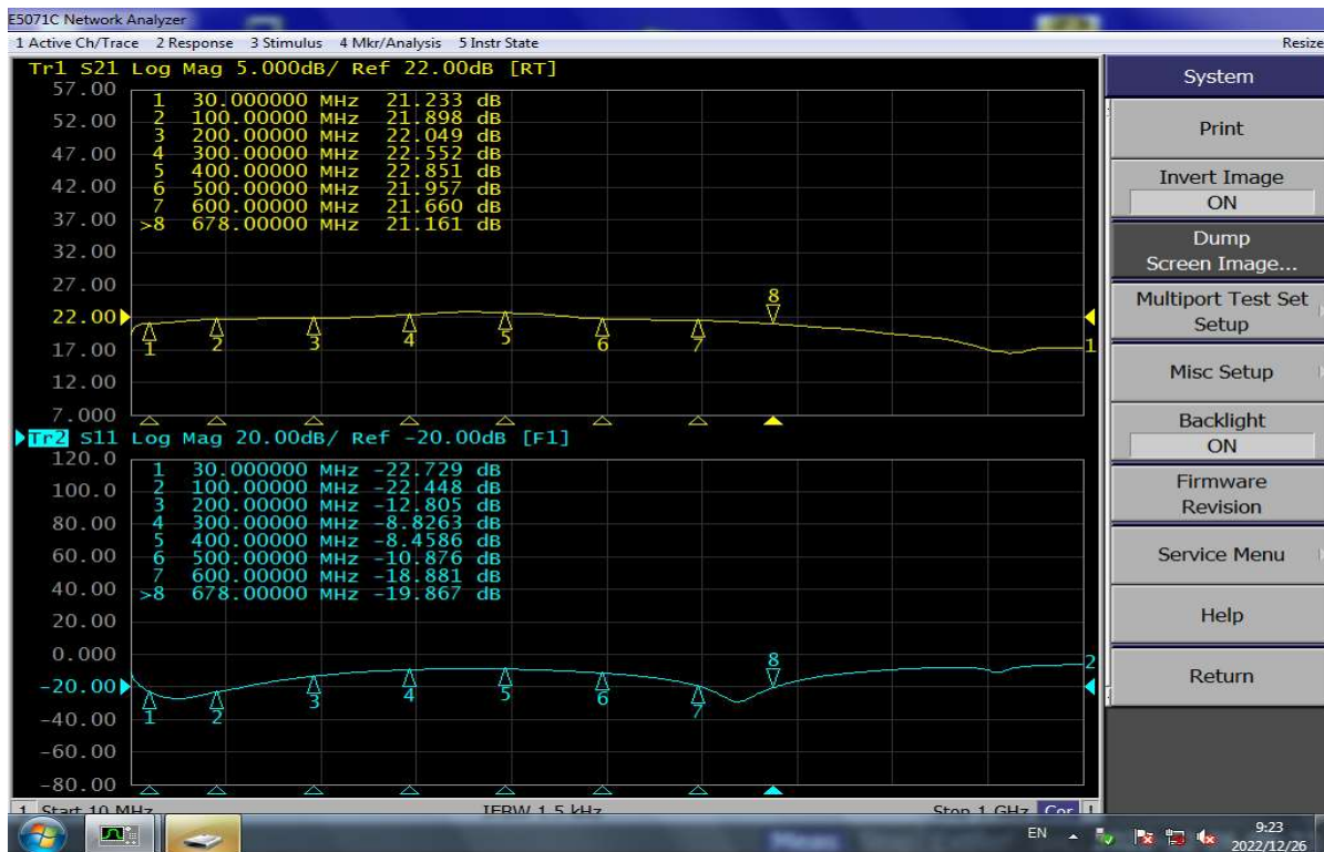
Figure 1: Network analyzer output, S11 and S21 (VDD=28V IDQ=500mA)
