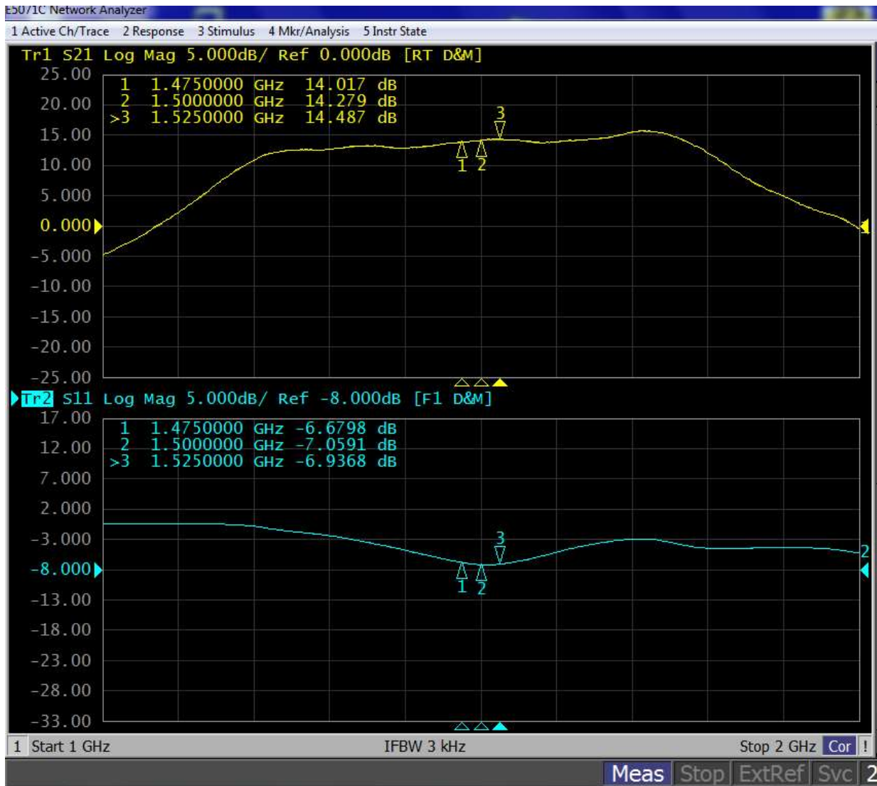
Figure 3. Network analyzer output S11/S21
