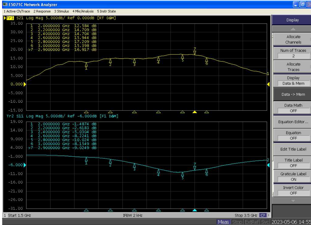
Figure 3. Network analyzer output S11/S21 (VDS=28V IDQ=200mA VGS=2.95V)
