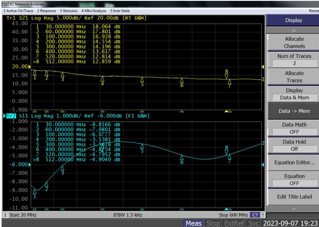
Figure 1: Network analyzer output S11/S21 at 28V Idq=450mA
