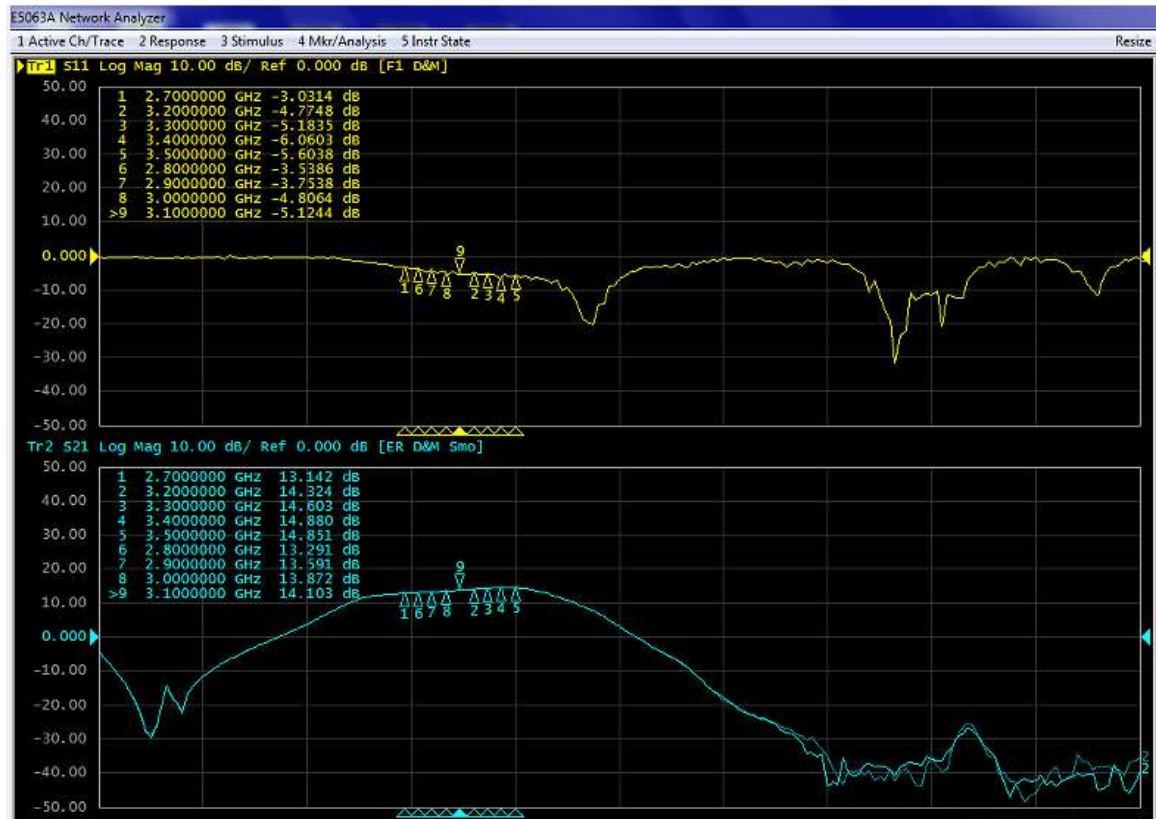
Figure 4. Network analyzer output S11/S21
