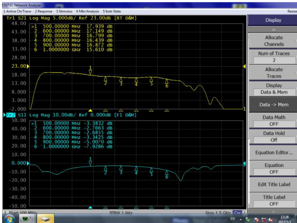
Figure 1: Network analyzer output, S11 and S21
