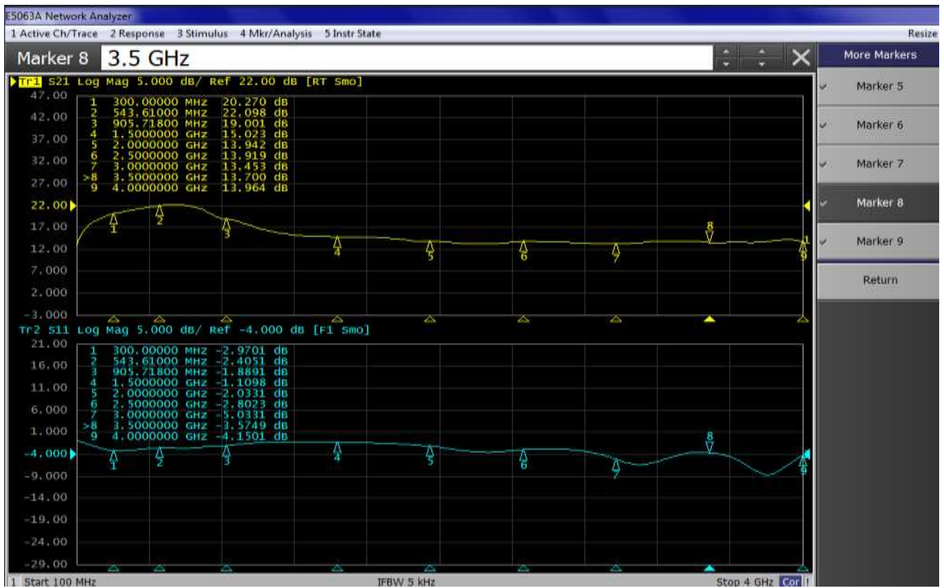
Figure 2: Output of network analyzer S11, S21 V_{GS} = -2.4\text{V} , V_{DS} = 32\text{V} , I_{DQ} = 130\text{mA} , input power = 0dBm
